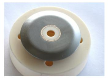
Active-brazed focus electrode made of  $\rm Al_2O_3$  ceramic and tantalum (Listemann AG, Eschen/LI)
