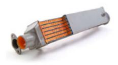
Exhaust gas heat exchanger made of stainless steel with nickel base brazing material, brazed in a vacuum, high temperature procedure (pattern) (Modine Europe GmbH, Filderstadt
